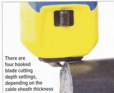
When closed, the hooked blade is concealed and covered by a cap. The blade must be released manually
